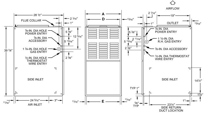
**NOTES:** 1. Two additional %-in. dia knockouts are located in the top plate.
